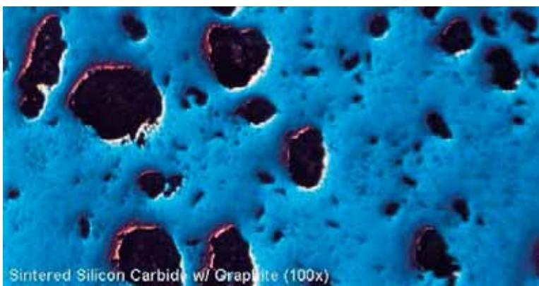
Figure 1. Graphite-loaded sintered SiC structure
