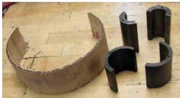
Figure 2. Tamping tools: split tubing, metallic bushings, cardboard
