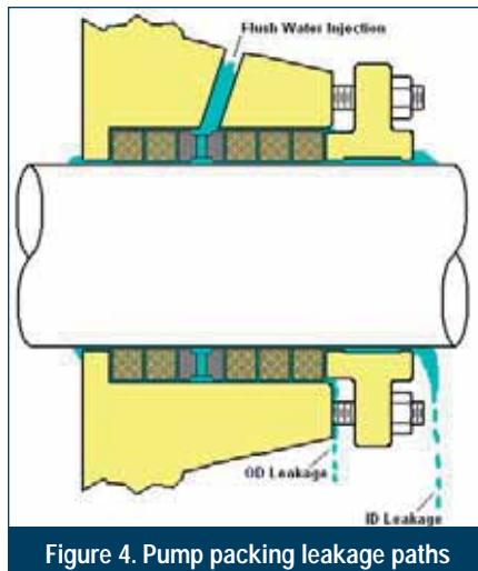
Figure 4. Pump packing leakage paths
