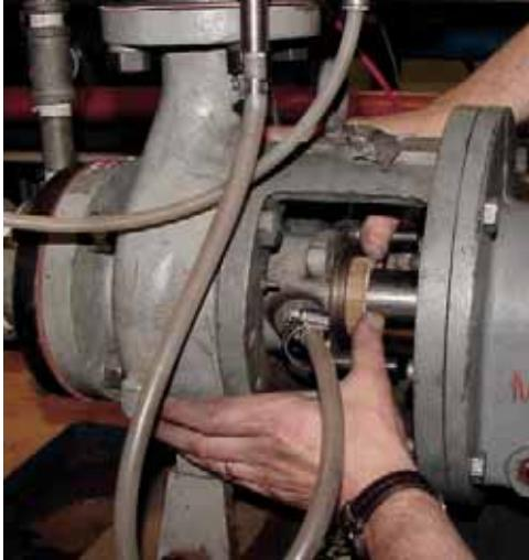
Figure 3. Using cardboard tamping tool
