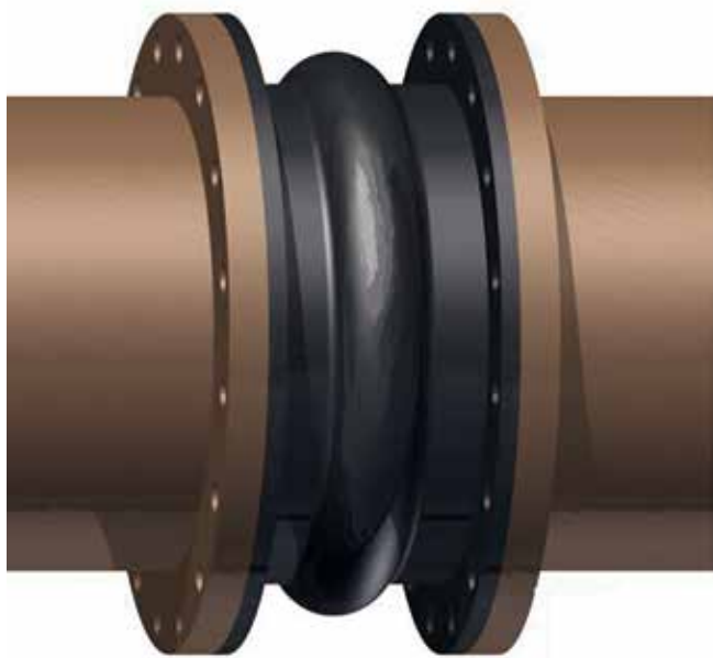
A typical expansion joint (Article images courtesy of FSA.)
