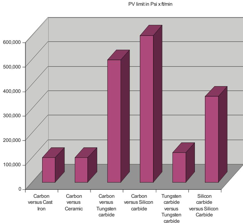
**Figure 2. Nominal PV limits for typical face materials in non-lubricating fluids.**
