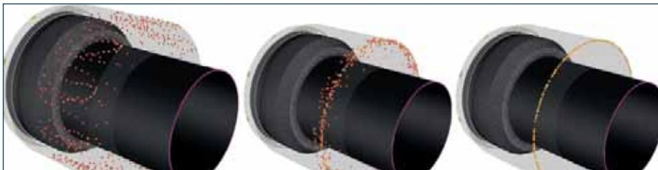
Figure 2. Time progression showing solids concentrating at bore.
