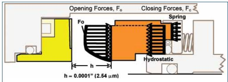
Figure 2. Forces on gas seal faces
