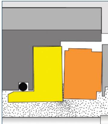
Figure 1. Solids migration into seal face gap
