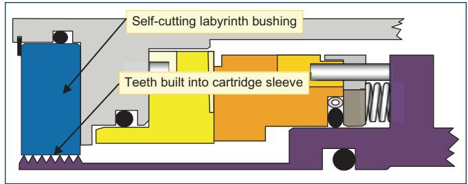
Figure 3. Typical labyrinth seal design feature
