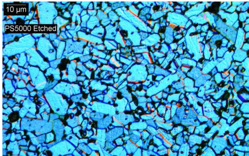
Figure 2. The grain structure of sintered silicon carbide.
