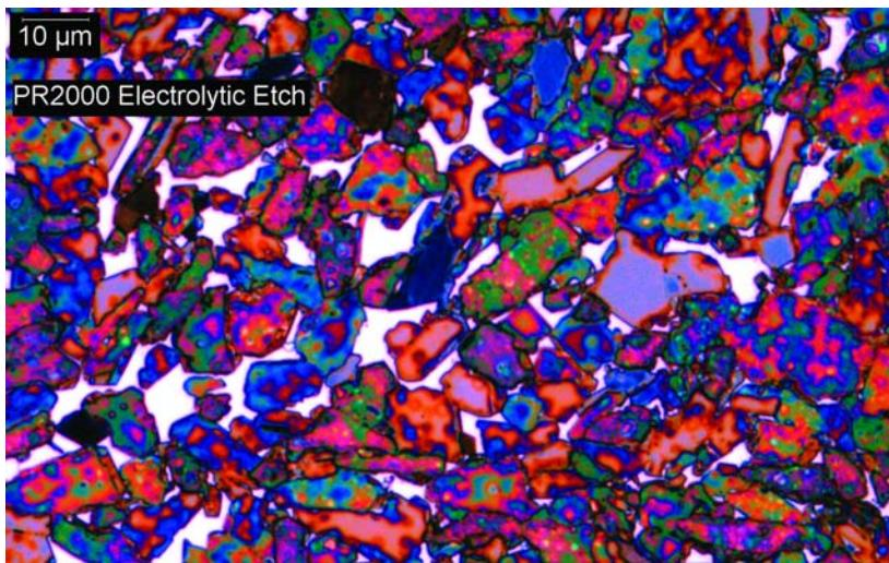
**Figure 1.** The grain structure of reaction bonded silicon carbide with free silicon.
