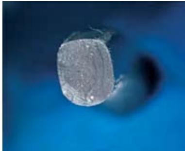
**Figure 1. Cross section of O-ring showing compression set.**
