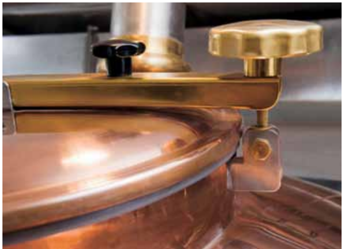
Figure 1. PTFE gasket on brewery kettle
