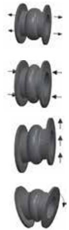
Figure 2. Axial extension and compression (in inches), lateral or parallel movements (in inches), and angular movements (in degrees).
