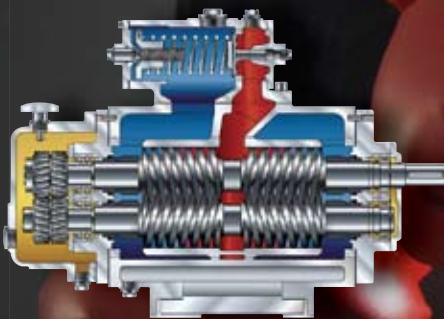
Leistriz' twin-screw flare knock-out pumps are perfect for corrosive, abrasive, or flammable liquids and operate trouble-free, even when confronting entrained gases.
