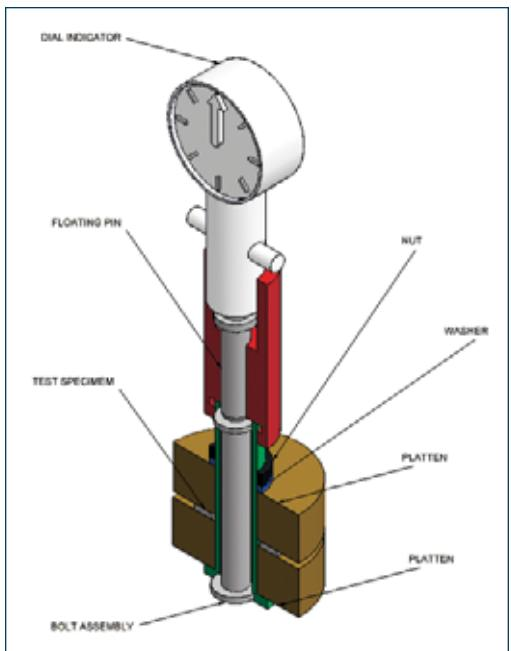
Figure 3. ASTM F38 Method B Relaxometer
