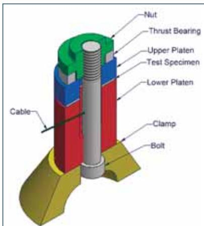
Figure 2. ASTM F38 Method A Relaxometer
