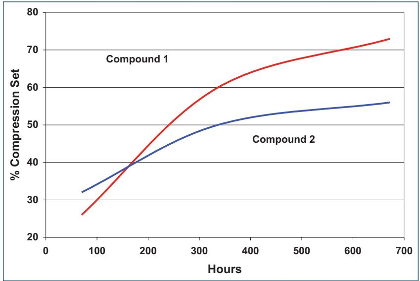
Figure 1. ASTM Method D395, 204°C, AS-568 214 O-rings
