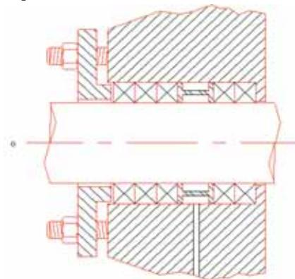
**Figure 1.** Diagram of a typical packing stuffing box flush system.
