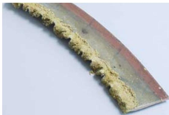
**Figure 1. Non-metallic gasket showing chemical attack.**
