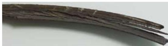
**Figure 2. Fiber gasket showing over compression.**
