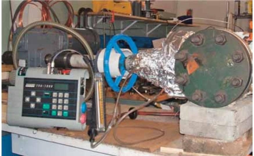
Figure 3. API 624 test device
