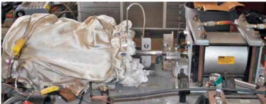
Figure 2. API 622 test device
