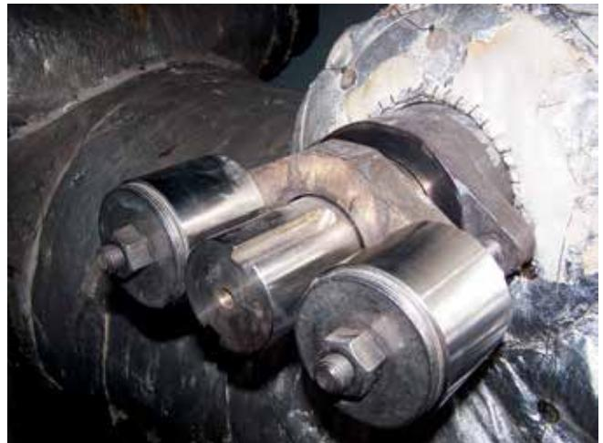
Figure 2. Live loaded assembly
