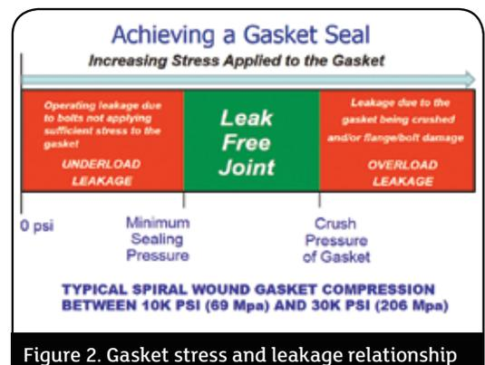
Figure 2. Gasket stress and leakage relationship
