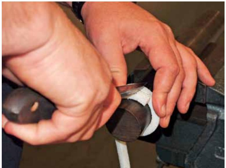
**Figure 1. Cutting on a mandrel**
