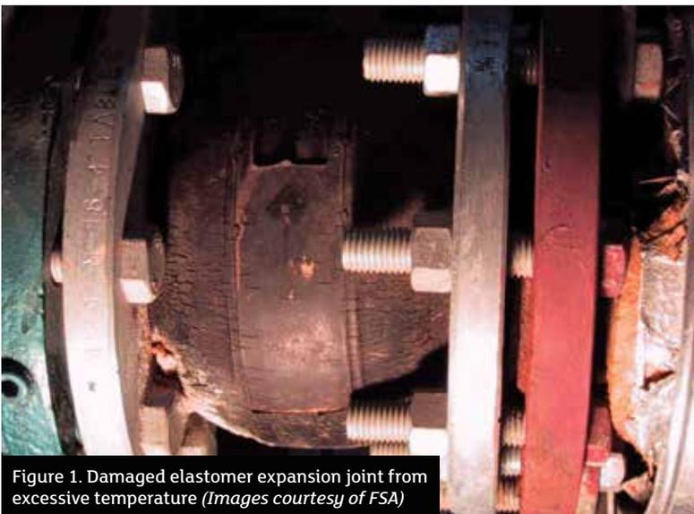
Figure 1. Damaged elastomer expansion joint from excessive temperature (Images courtesy of FSA)
