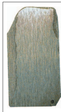
Figure 3. Binder leaching in tungsten carbide insert.
