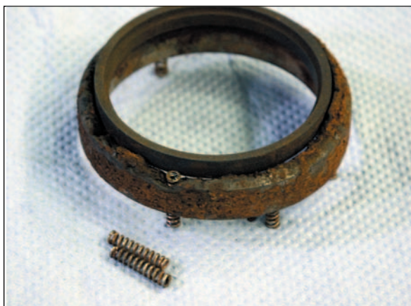
Figure 1. Signs of chemical attack on mechanical seal
