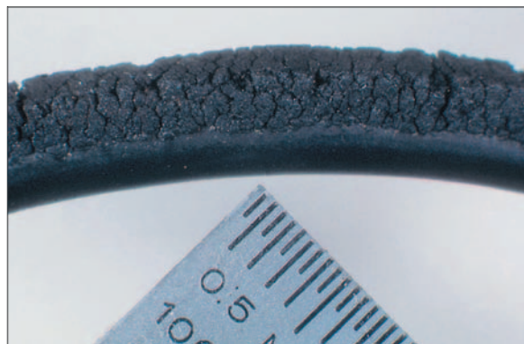
Figure 2. O-rings exhibiting symptoms of chemical attack (courtesy of DuPont Dow Elastomers)
