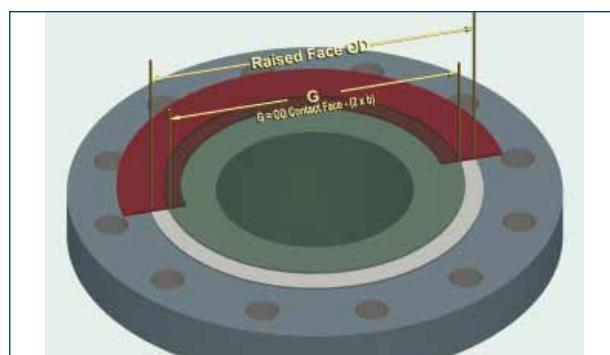
Figure 1. Load reaction Diameter G
