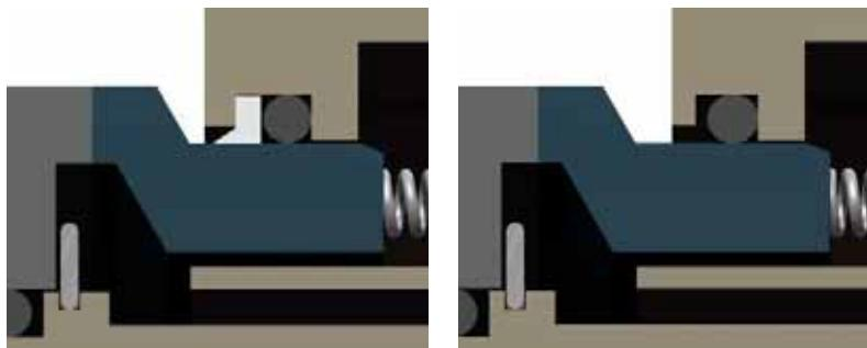
Figure 2. O-ring groove designs (right); wiper ring design (left).
