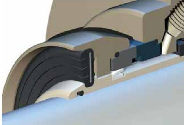
Figure 3. Mechanical seal design using a cone spring.
