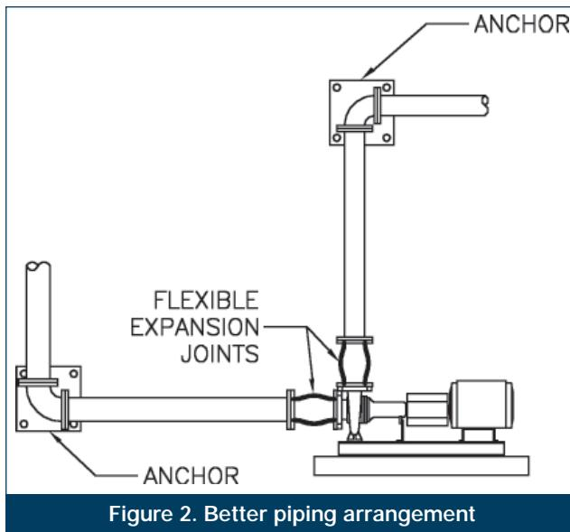
**Figure 2. Better piping arrangement**
