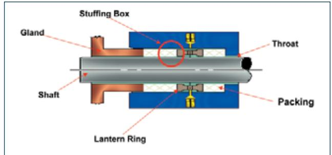
Figure 2. Typical stuffing box
