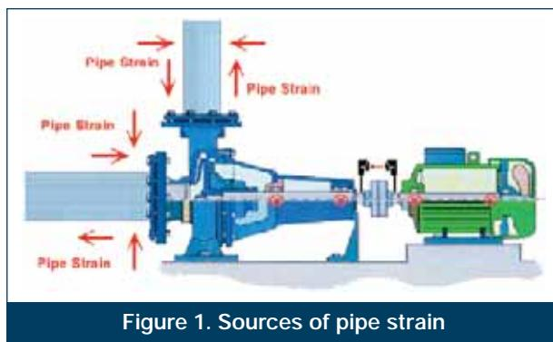
Figure 1. Sources of pipe strain
