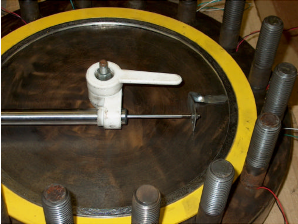
Figure 4. Radial Measurement of Gasket Inside Dimension Using Ratcheting Mechanism for Positioning (top flange removed for photograph)
