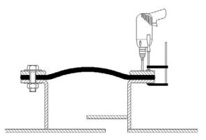
NB It is <u>very important</u> that the clamps (on both sides of the hole) hold the material securely otherwise the fabric and the insulating materials may rotate with the drill, resulting in tearing.
