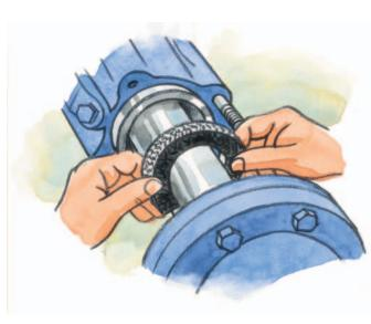
After last ring is installed, draw gland up evenly until nuts are finger-tight.
