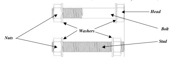
The function of the fastener is to clamp the joint sufficiently to prevent slip or leakage, and hence it must be strong enough to support the tension induced on initial tightening, together with the additional loads it will endure in service (as a result of
