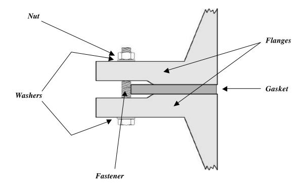
Only when all the components of the system are working together in harmony can the seal be expected to provide a good performance over a reasonable lifetime. The integrity of a safe seal depends upon:
