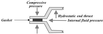
So, the primary function of a gasket is to create and maintain a seal between flanges, under conditions which may vary markedly from one joint to another, dependent upon the nature and type of application. To meet these varying conditions, a number of flange / fastener / gasket systems have been developed, and many factors must be considered when selecting the most appropriate assembly, including:
