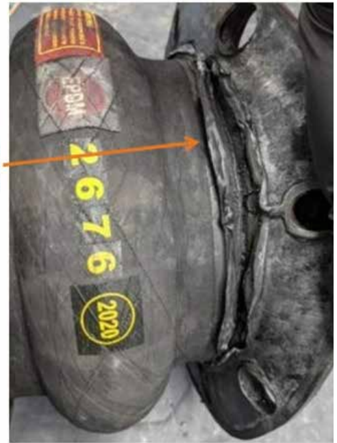
IMAGE 4: Cycle life testing failure
