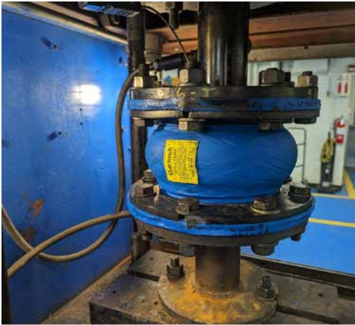
IMAGE 3: Performance expansion joint under destructive durability testing
