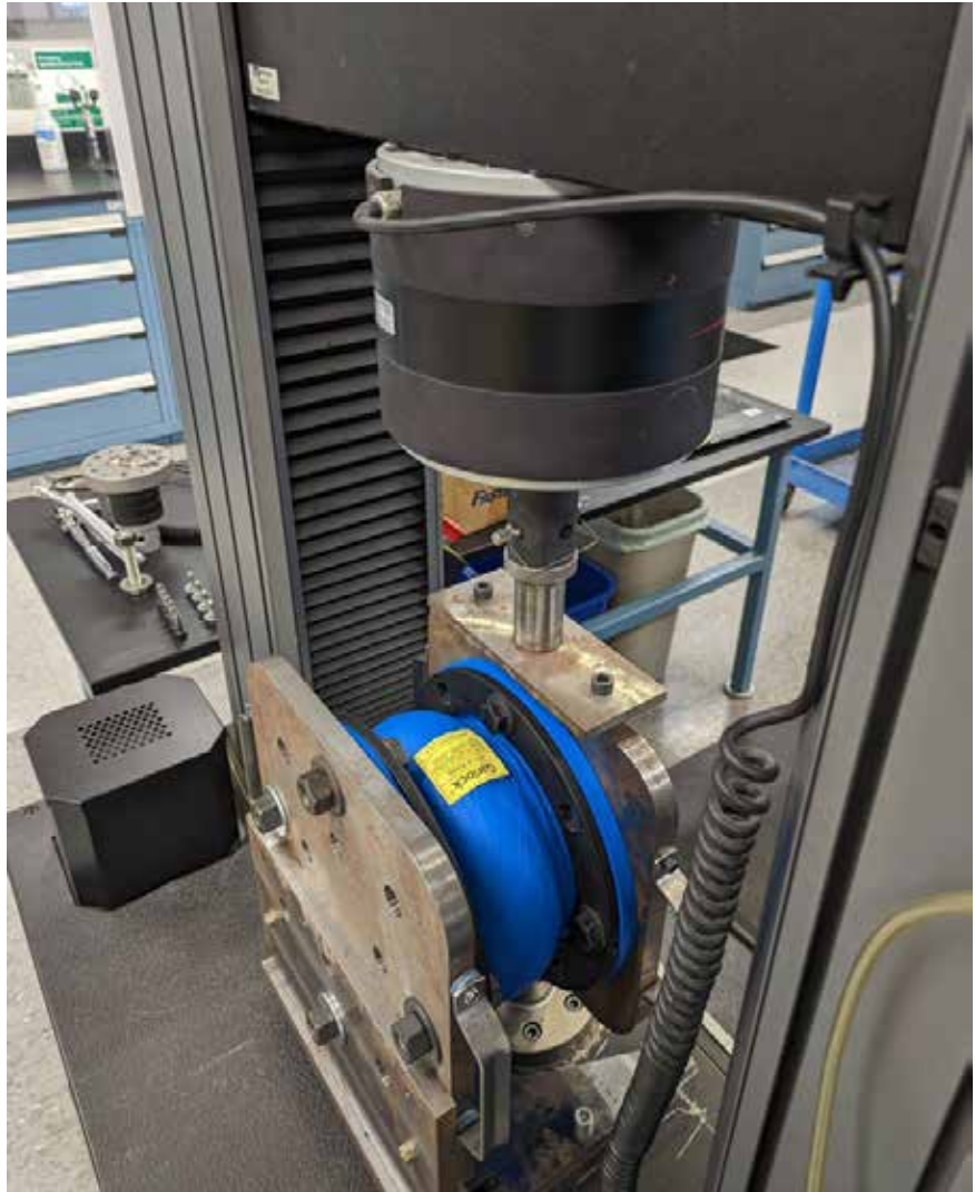
IMAGE 1: Performance expansion joint spring rate validation testing (Images courtesy of Garlock)
