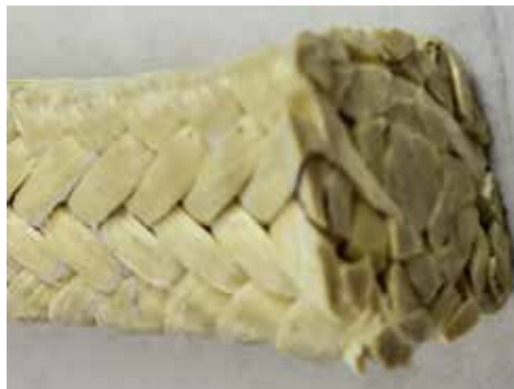
IMAGE 1: The unraveling or fragmentation of packing material after it undergoes the cutting process (Images courtesy of A.W. Chesterton Company)
