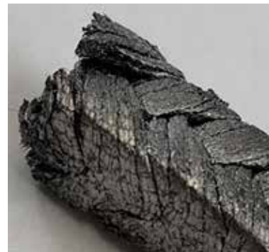
IMAGE 1: The unraveling or fragmentation of packing material after it undergoes the cutting process (Images courtesy of A.W. Chesterton Company)
