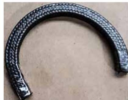
IMAGE 2: The practice of taping the ends of cut rings and lengths
