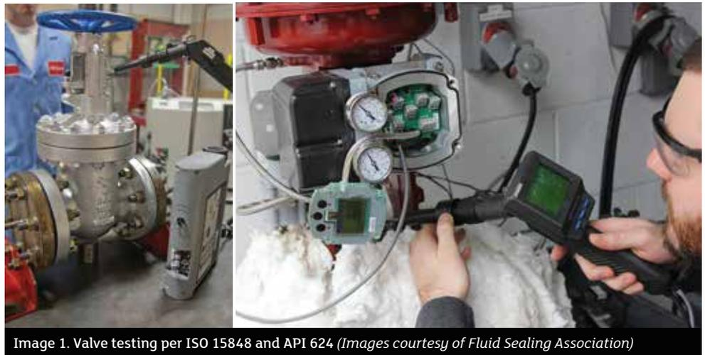
Image 1. Valve testing per ISO 15848 and API 624 (Images courtesy of Fluid Sealing Association)
