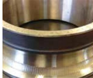
Helwig's Bearing Protector extends the life of motors by keeping shaft voltage to a minimum. Prevents pitting and costly damage to bearings. The best choice for the motor industry.
