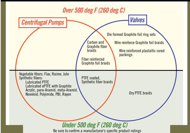
of its low coefficient of friction, wide chemical compatibility, low leak rate, long life and suitability for a broad range of applications as a general-purpose packing (see Figure 2).
