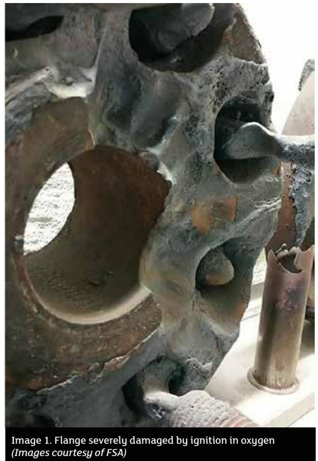
Image 1. Flange severely damaged by ignition in oxygen (Images courtesy of FSA)
