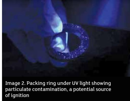
Image 2. Packing ring under UV light showing particulate contamination, a potential source of ignition
