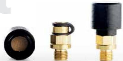
For venting the electrical gear motors in a clean and reliable manner. Unique construction against moisture and dirt. Opening pressure 0.15 - 0.25 bar. 100% tested thanks to a fully automated assembly. Assembled transportation lock and dust cap possible.
