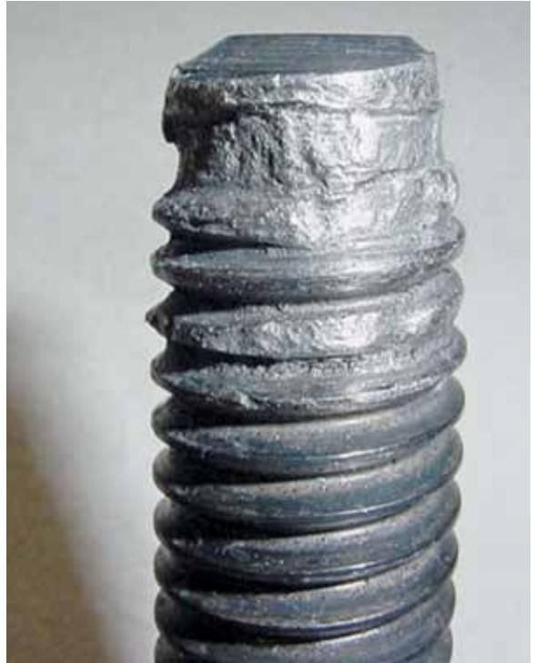
Figure 1. Galled stainless steel bolt
