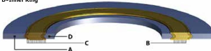
used in place of soft filler material and may have a soft surface layer of material such as flexible graphite. The primary seal against leakage is the inner metal overlap, where the density of the gasket is the greatest when compressed.
