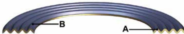
Figure 2. A=Metal Jacket (Outer Layer) B= Filler Material
