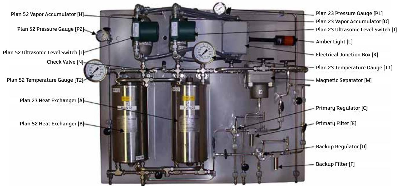
IMAGE 6: Typical auxiliary support system (panel) for Plan 23/52
