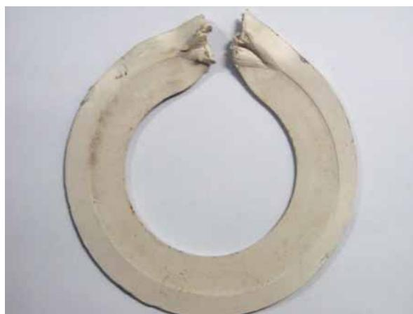
Figure 1. Gasket rupture from blow out
