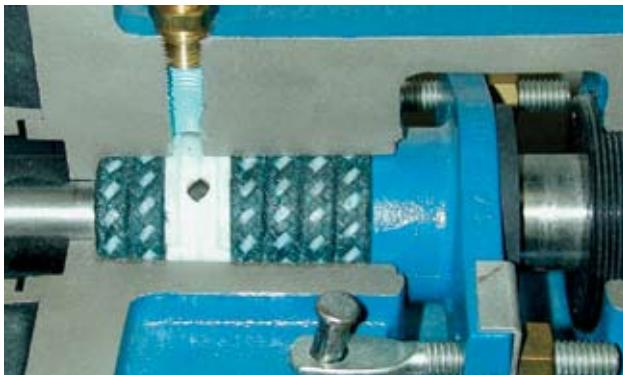
Figure 1. Cross section of a typical pump stuffing box installation.
