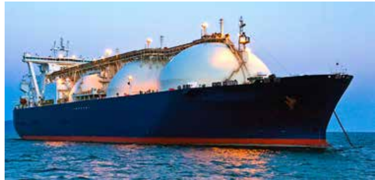
Image 1. Liquid natural gas must be liquified and cooled to ship. (Images courtesy of the author)
