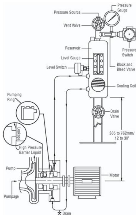
**Figure 1. Plan 53 Dual Pressurized Barrier System**
