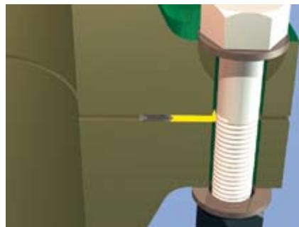
**Figure 2. Spiral wound gasket design with guide ring – flat face flange.**
