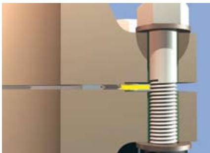
**Figure 1. Spiral wound gasket with both guide & inner rings – raised face flange.**
