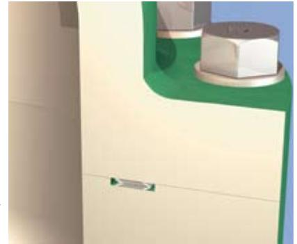
**Figure 4. Spiral wound gasket design for recessed flange groove.**
