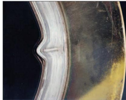
**Figure 3. SWG with buckled inside diameter**
