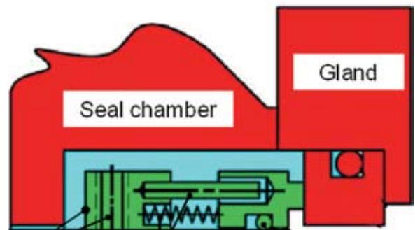
**Figure 1. Cross-section of a typical mechanical seal assembly.**
