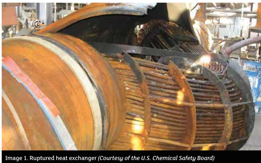
Image 1. Ruptured heat exchanger (Courtesy of the U.S. Chemical Safety Board)
