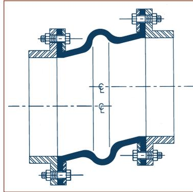
**Figure 3. Lateral offset built into expansion joint**
