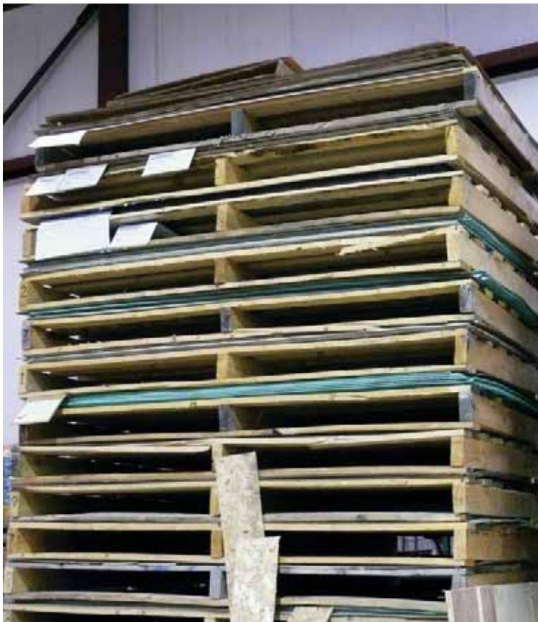
Figure 2. Flat storage of sheet gasket material
