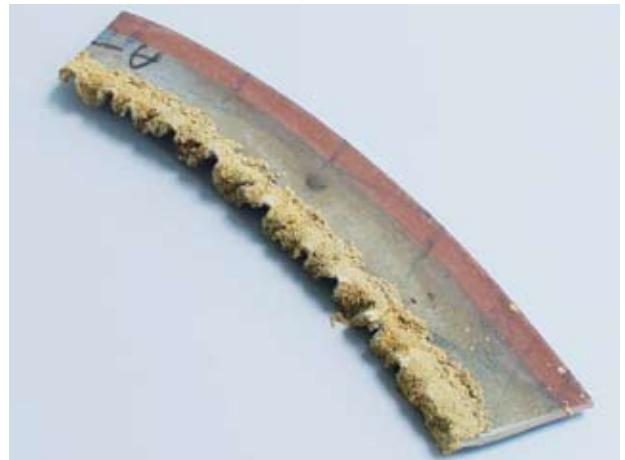
**Figure 1. Gasket showing chemical attack.**
