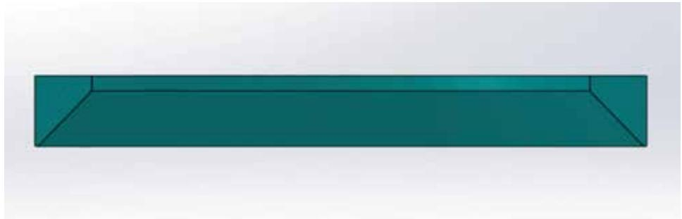
The structure of a metal seal consists of a wider top, an angle consisting of 45 degrees or 30 degrees and a wire-thin toe at the bottom.
